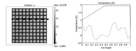
Figure 8-3: Equation 8-3 solved using unstabilized Galerkin formulation. The right plot compares the unstabilized solution (dashed line) along the dashed line in the left plot (y = 0.8) with the reference solution (solid line).
