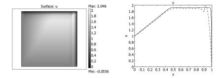
Figure 8-5: Equation 8-3 solved using streamline diffusion. The right plot compares the stabilized solution (dashed line) along y = 0.8 with the reference solution (solid line).
