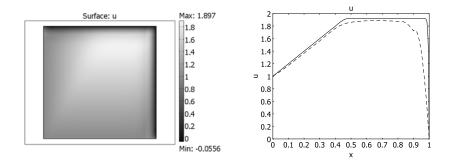
Figure 8-6: Equation 8-3 solved using streamline diffusion and crosswind diffusion. The right plot compares the stabilized solution (dashed line) along y = 0.8 with the reference solution (solid line).
