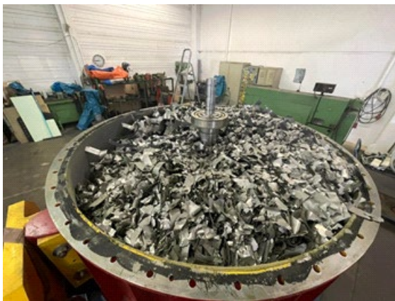
Figure 3: Disintegrated steel strip spiral without damage of the outer housing.
