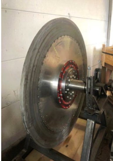
Figure 2: Flywheel configuration with the spiral steel strip segment, the aluminum core, and shaft.
