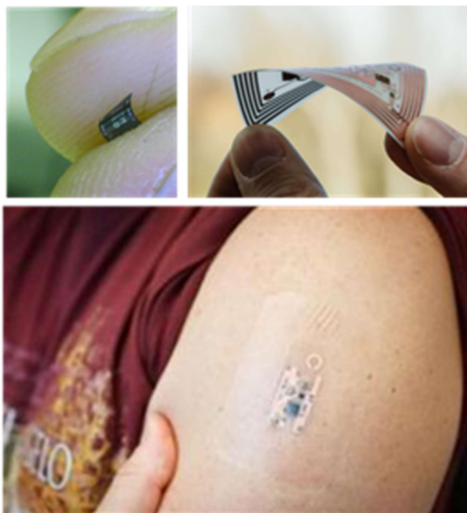
Figure 1. Thin chip and skin sensor patch developed at Holst Centre
