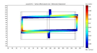
**Figure 1**: Representative volume element of masonry and effective plastic strain of elastoplastic mortar.
