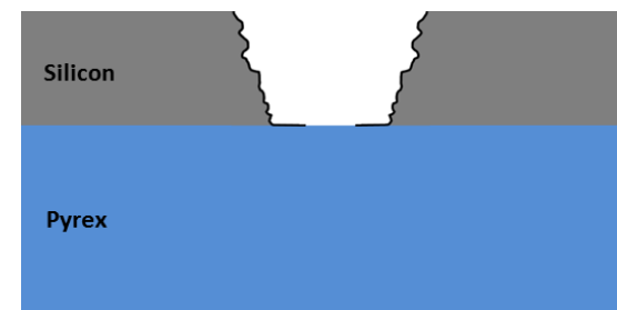
Figure 7: Qualitative View of Pyrex-silicon Bonding Fracture
