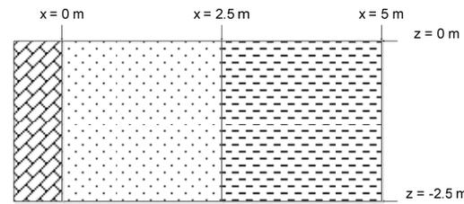
**Figure 4.** Synthetic model of a concrete impermeable wall (left), with backfilled sand (middle) and the untouched subsoil (right).
