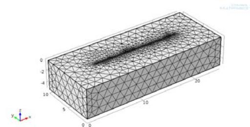
**Figure 10.** COMSOL resistivity model with meshing and electrodes.
