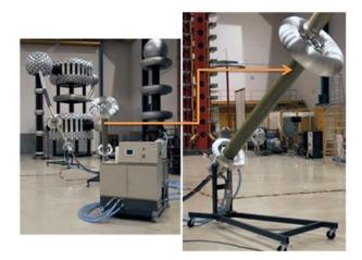
**Figure 1**: The Cable Termination (CaTr)- Right and CaTr System being used in high-voltage AC test system- Left.
