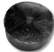
Figure 2. Single grain YBCO cylinder (www.can.cz)
