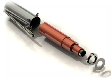
Figure 7. Exploded view of magnet assembly for the DDH coils of Figure 6. The SS housing with inlet and outlet water cooling tubes are shown.
