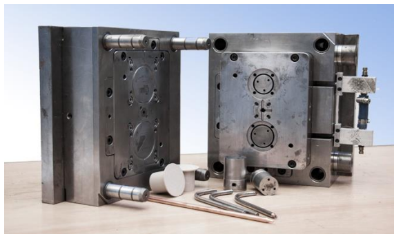
Figure 1 Heat pipe tempered mould
