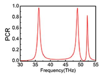
**Figure 1**: Triple bands(36.15, 48.95 and 52.20 THz) of cross-polarization conversion is achieved.
