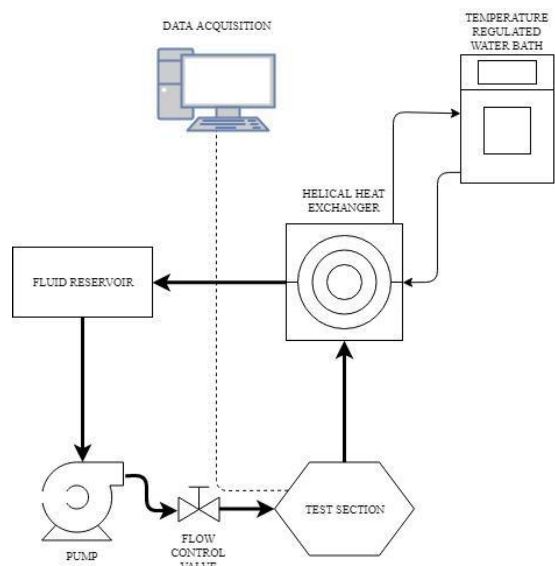
Figure 1. Schematic of Experimental Apparatus
