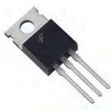
Figure 1. TO-220 transistor package.
