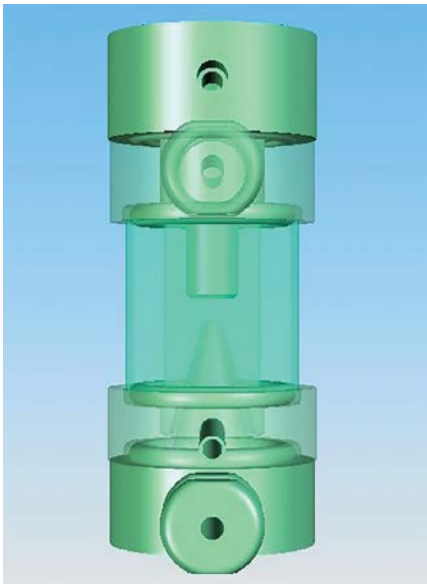
FIGURE 4 CAD model of the micro aperture-electrode system, which was imported into COMSOL Multiphysics using the CAD Import Module.
