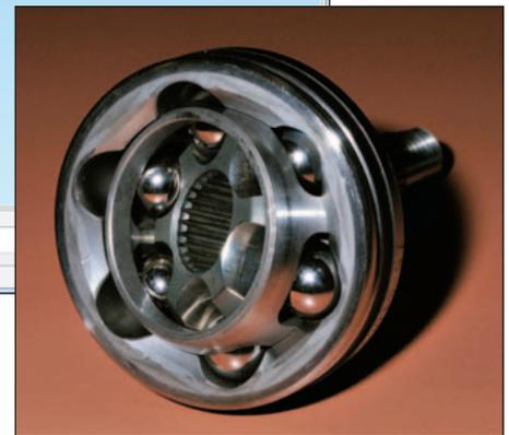
Figure 2. A Rzeppa CV joint (right) and the simulation (above) showing the final configuration and the absolute displacements of the joint when the shaft reaches the maximum angle with respect to the original configuration.
