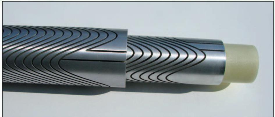
Figure 1. 2-layer multipole DDH magnet.
