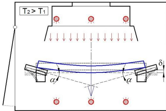
Figure 2: Modified windscreen forming process.
