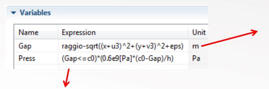
If 'Gap' becomes lower than the defined parameter c0 (= 1e-5 m) a pressure variable 'Press' is generated on the outer surface of the shell-catheter, according to a standard contact algorythm (with penalty factor).
