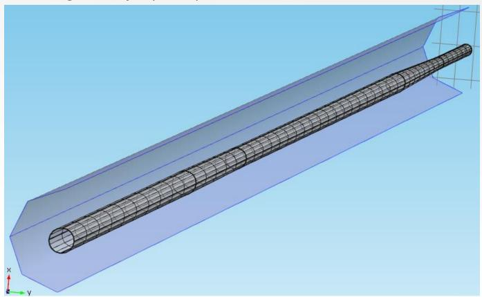
The outer tube is for representation purposes only, since <u>no contact can be</u> <u>defined with SHELL elements</u>
