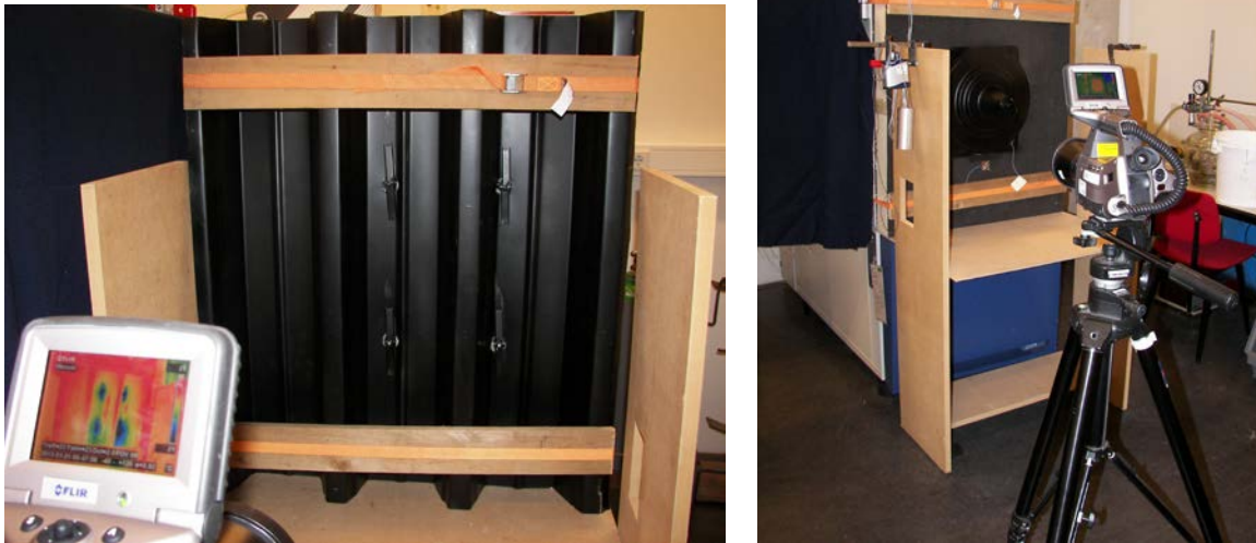
Figure 3. Measurement set-up of the roofing system with anchor, mounted at the front opening of a climate cabinet
