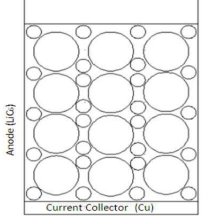
Figure 1: 2 D-Model of Li-Ion Cell.
