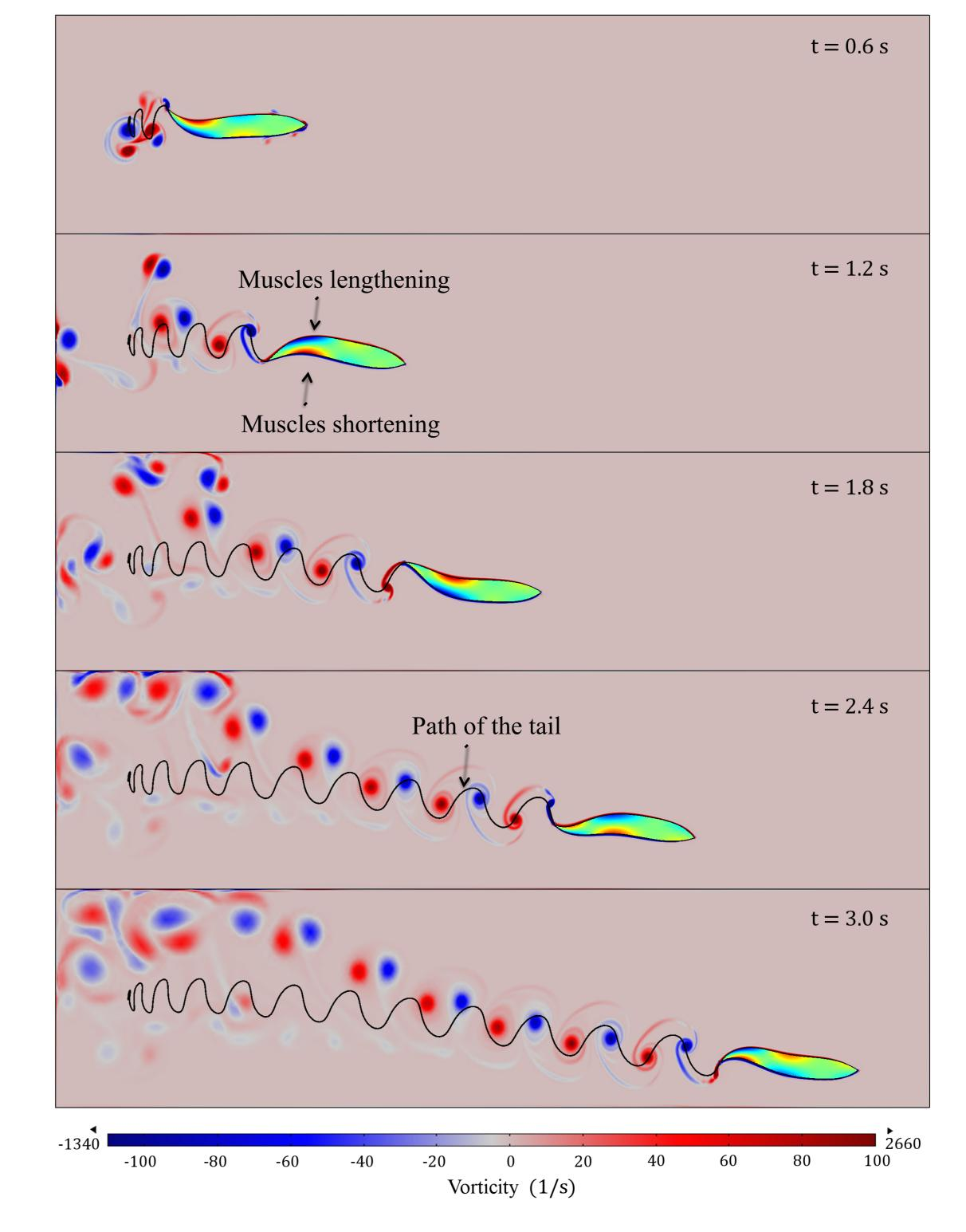
Snapshots of fish swimming with fluid velocity (left) and vorticity (right); muscles stroke (red colored) bends the fish and produces the swimming thrust. A long wake lies behind the fish.
