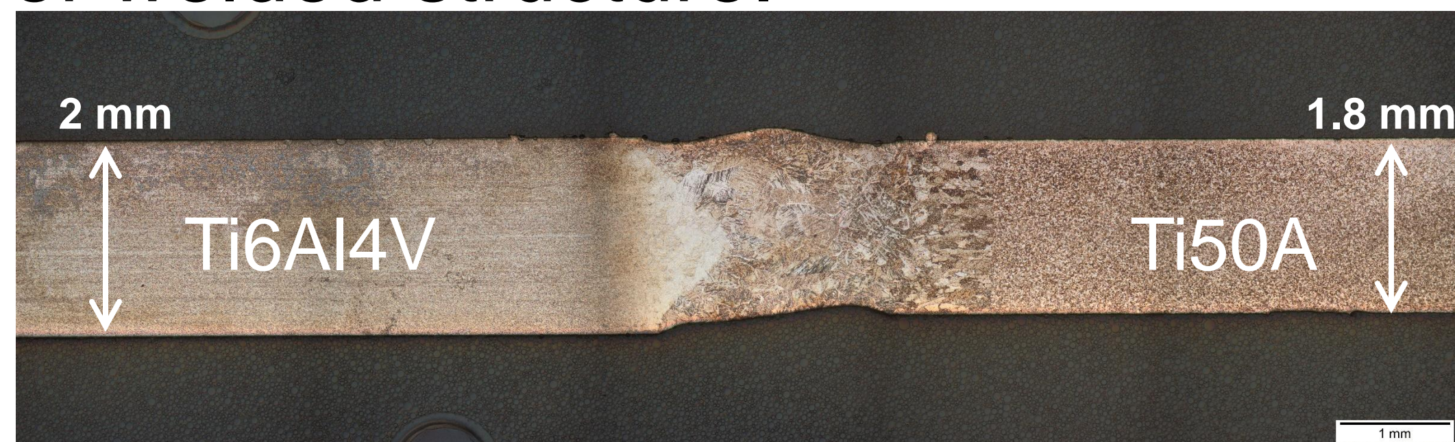
Figure 1. Cross-section of a Laser welded flat joint (Welding Speed = 2 m/min, Laser Power = 2 kW)
