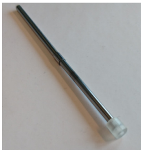
Figure 7. A metal tube with an insert in the middle and a printed part at one end for receiver attachment.
