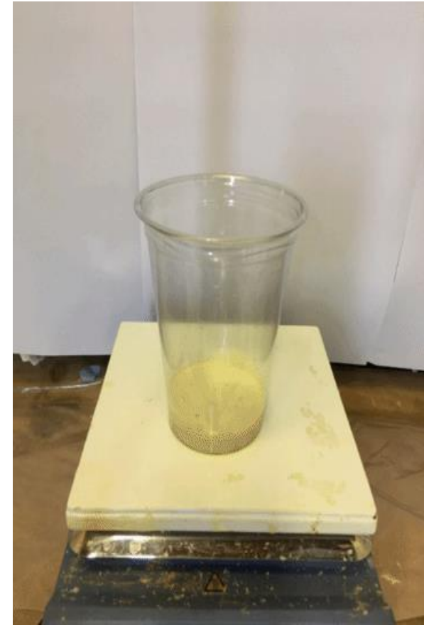
Animation of polyurethane foam expansion. The animation spans approximately 30 minutes.
