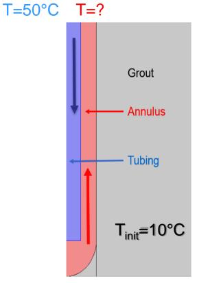
• The fluid flow was first solved in a stationary study and the resulting pressure and velocity fields were used in heat transfer study
