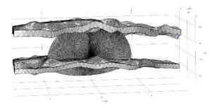
• heat transfer in a fracture is similar to porous media
