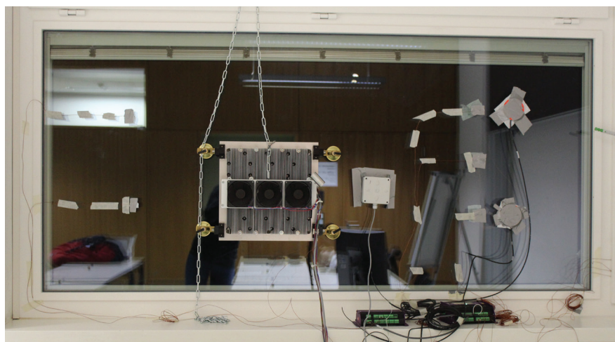
FIGURE 2. Setup at the Living Labs of the Free University of Bozen-Bolzano, including two heat flux plates, an in situ device designed by the University of Innsbruck to measure the overall heat flux, and several thermocouples for the surface and air temperature measurement.
